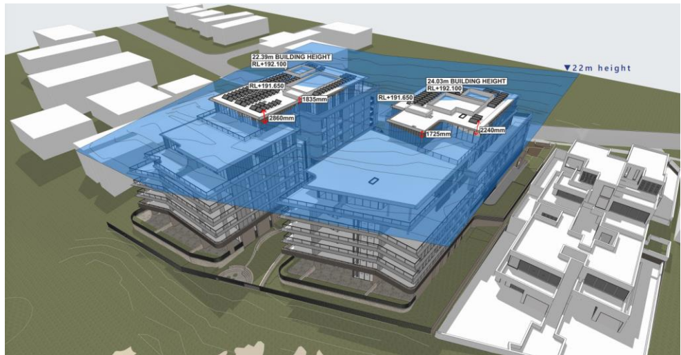
Figure 7 Proposed Variation to the 22m Height of Building development standard Source: Plus Architecture
